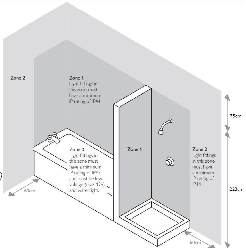
THIS LIGHT FITTING IS IP44 MAKING IT SUITABLE FOR ZONES 1 AND 2
